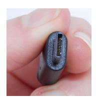
On the right side of Vario 464 you can find the USB port, which is USB type C. Special about the USB Type C port is, that it doesn't matter which direction the USB plug is facing. No more finding the right position of the plug.
